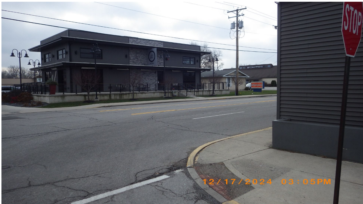
Figure 3. Looking west from approximate standard stopped position on Denver Street, with inadequate sight distance to the west.
