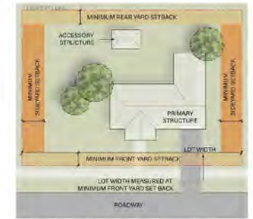
Example of minimum setback and lot width measurements.
